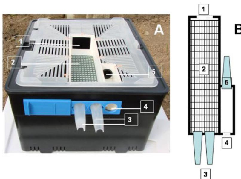
**Figure 1.** The newly developed two-way dispenser. (A) Photograph from the front without the cover lid, and (B) schematic drawing, top view. (1) Connection of the exit compartment to the bumblebee hive; (2) exit compartment with a grid at the bottom that contains the powder MCA formulation; (3) exit holes with bumblebee-in-closer; (4) entrance hole; (5) bumblebee-in-closer, connecting the entrance compartment to the bumblebee hive. Dispenser length 20 cm.
